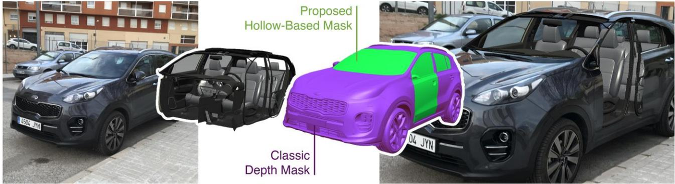
Figure 1: The proposed occlusion system. A real object (left) is augmented (right) with virtual content through the use of an inverse hole-based depth mask, shown with green color, instead of the traditional one, depicted in red color (middle).
